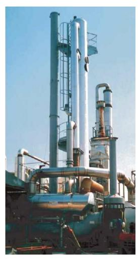
Gas combustion plant. Incineration of gas streams coming from solvent polluted water stripping plant.
